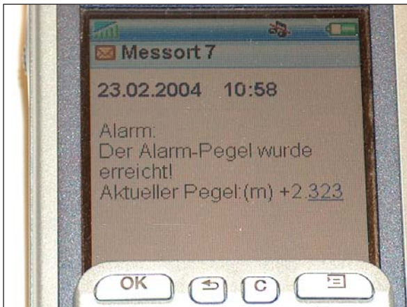
GSM-1 sends an alarm signal to a mobile telephone or an evaluation system
